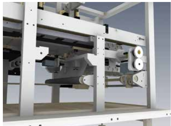
The PowerDRIVE controls the adjustment of the height and the turning of the molds in the demolding station.
