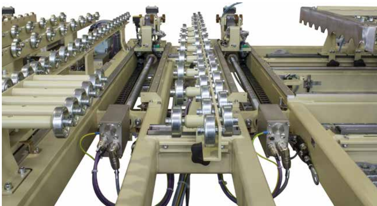
Eight positioning drives automatically and precisely place the stop systems in position.
